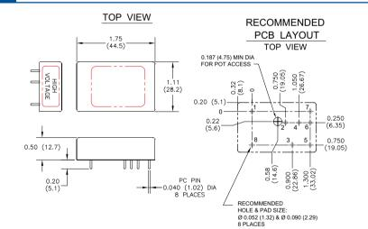
5Vin 12Vin Pin Function Description VOUT High Voltage Output Ground to Pin 8 1 2 VPGM Voltage Programming Input, <150uA 0 to +2.048V 0 to +5V 3 SGND Signal Ground [For VPGM, VIN, VMON] Low Voltage Ground Voltage Reference Output, +/- 1% , 1 mA 4 VREF +2.048V +5V 5 CGND Case Ground Case Ground VIN Input Voltage +4.75 to +5.25V +11.5V to +15.5V 6 7 VMON Voltage Monitor Output, 1mA, scales to 0 to 100% Vout 0 to +2.048V 0 to +5V 8 HV RTN HV Output Return Ground for Pin 1
