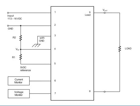
Operate with 5VDC Reference Voltage Variable output
