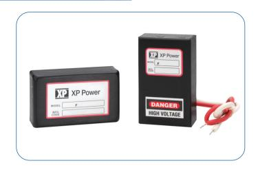
The F Series is a broad line of robust, field-proven DC to HV DC converters which deliver 10 Watts continuous output power. Outputs range from 100V to 12kV. The input and output are galvanically isolated so a unit can be used to deliver a positive or negative high voltage output. The output voltage is proportional to input voltage with a low 0.7V typical turn-on voltage.
