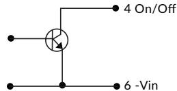
Positive logic: "On" if pin 4 is high >3.5V to 160VDC
