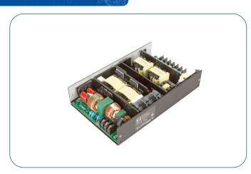
Approved for medical and ITE applications, this range of convection cooled single output AC/DC power supplies are packaged in an ultra compact foot print of just 5.0" by 8.0". The UCH600 provides up to 600 W convection-cooled leading to very high power density of 9.5 W/in<sup>3</sup>.
