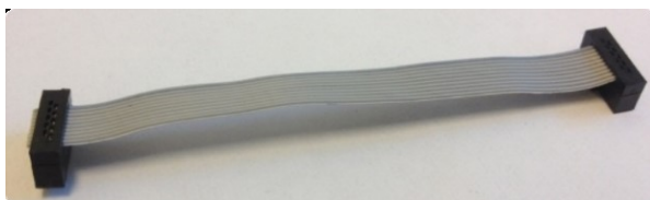
Figure 13: Standard ribbon cables can be used for connecting the MTi OEM to another board
