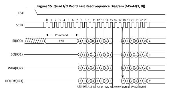
Figure 16. Quad I/O Word Fast Read Sequence Diagram (M5-4= (1, 0))
