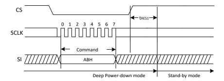
Figure 25. Release Power-Down Sequence Diagram
