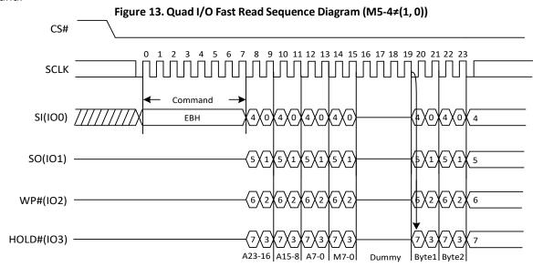
Figure 14. Quad I/O Fast Read Sequence Diagram (M5-4= (1, 0))
