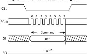
Figure 4. Write Disable Sequence Diagram
