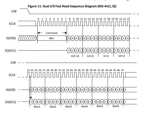
Figure 12. Dual I/O Fast Read Sequence Diagram (M5-4= (1, 0))
