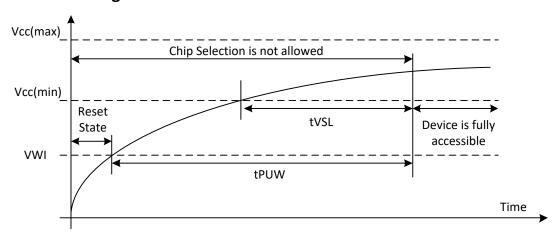
Table3. Power-Up Timing and Write Inhibit Threshold
