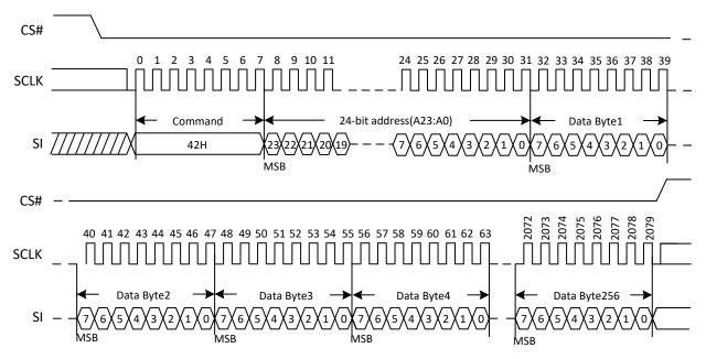
Figure 34. Program Security Registers command Sequence Diagram
