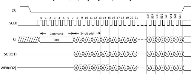
Figure 19. Quad I/O Page Program Sequence Diagram
