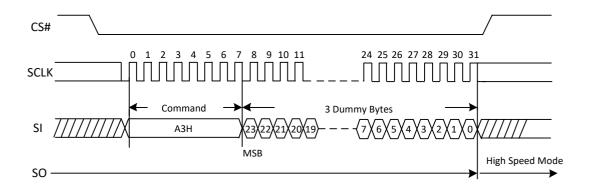
Figure 28. High Performance Mode Sequence Diagram
