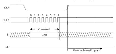
Figure 23. Program/Erase Resume Sequence Diagram
