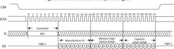
Figure 27. Read Identification ID Sequence Diagram
