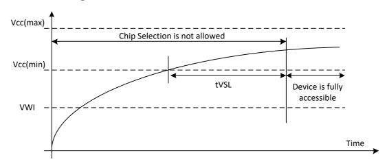
**Power-Up Timing and Write Inhibit Threshold**
