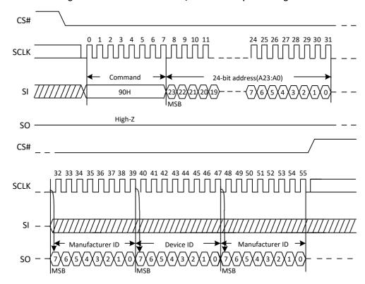
Figure 24. Read Manufacture ID/ Device ID Sequence Diagram
