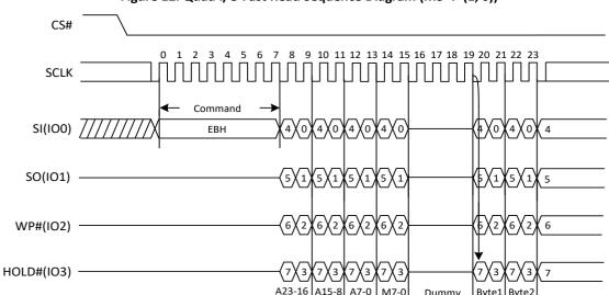
Figure 12. Quad I/O Fast Read Sequence Diagram (M5-4≠(1, 0))
