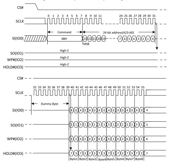
Figure 11. Quad Output Fast Read Sequence Diagram
