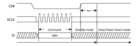
Figure 20. Deep Power-Down Sequence Diagram
