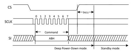
Figure 21. Release Power-Down Sequence Diagram
