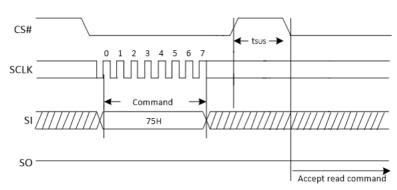
Figure 22. Program/Erase Suspend Sequence Diagram
