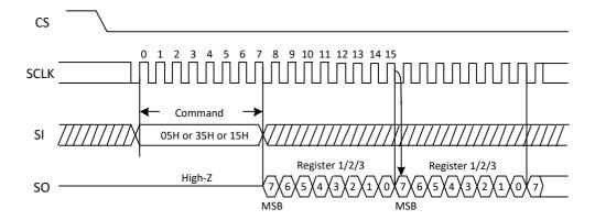
Figure 5. Read Status Register Sequence Diagram
