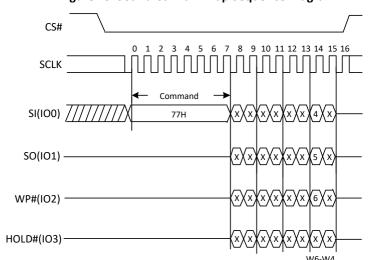
Figure 19. Set Burst with Wrap Sequence Diagram
