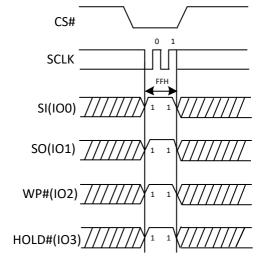
Figure 6a. Disable QPI mode command Sequence Diagram
