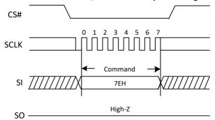
Figure 39a. The Global Block/Sector Lock Sequence Diagram (QPI)
