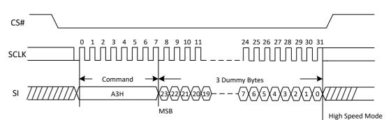
Figure 7. High Speed Mode Sequence Diagram
