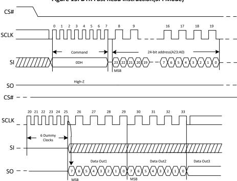
Figure 15. DTR Fast Read Instruction(SPI Mode)
