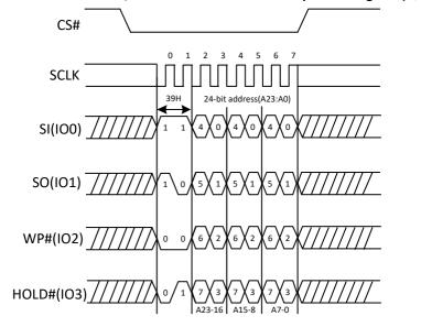
Figure 38d. Read Individual Block/Sector lock command Sequence Diagram
