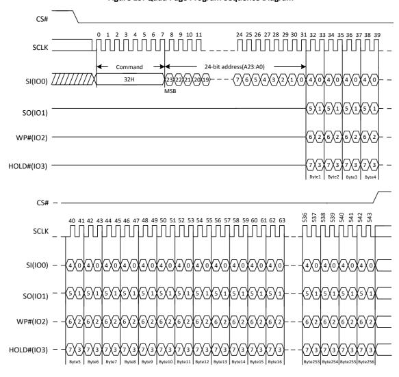
Figure 19. Quad Page Program Sequence Diagram
