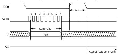
Figure 40. Program/Erase Suspend Sequence Diagram
