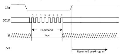
Figure 41. Program/Erase Resume Sequence Diagram
