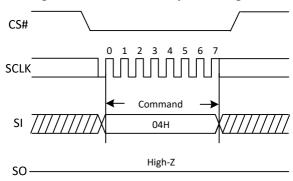
Figure 5a. Write Disable Sequence Diagram (QPI)
