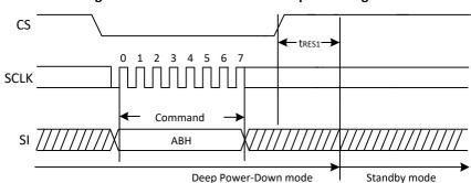
Figure 30. Release Power-Down Sequence Diagram
