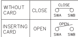
Circuit Diagram for Detect Switch
