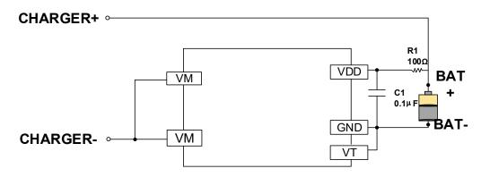
Figure 5 XB5332B in a Typical Battery Protection Circuit
