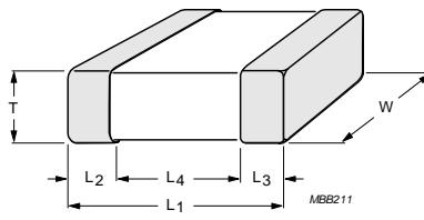
Fig. 2 Surface mounted multilayer ceramic c
