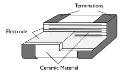
Surface mount multilayer ceramic capacitor construction
