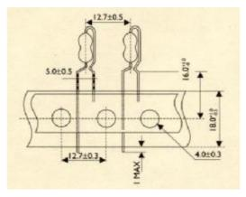
AV Type Forming for Taping (rated watts from 1/4W to 2WS applicable only )
