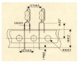
AV Type Forming for Taping
