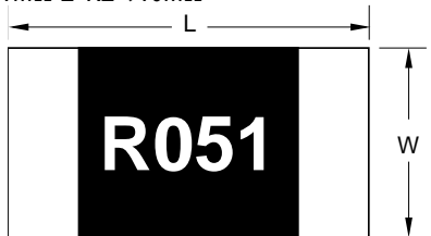
Fig. 5 Chip resistor outlines
