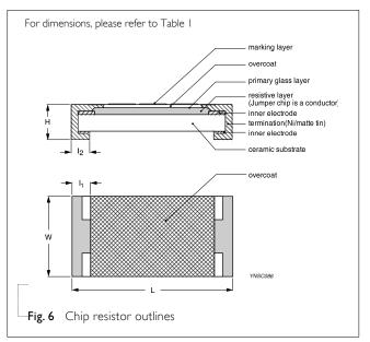
Chip Resistor Surface Mount RC\_L SERIES 0075 to 2512
