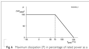
Fig. 6 Maximum dissipation (P) in percentage of rated power as a function of the operating ambient temperature (T<sub>amb</sub>)
