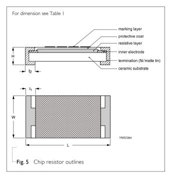
Chip Resistor Surface Mount RT SERIES 0201 to 2512 (RoHS Compliant)
