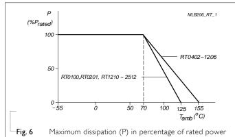
as a function of the operating ambient temperature (T<sub>amb</sub>)
