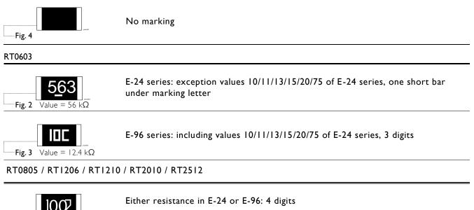
First three digits for significant figure and 4th digit for number of zeros
