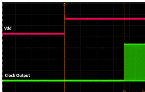
Figure 17. Startup Waveform vs. Vdd
