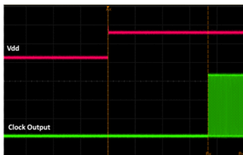
Figure 17. Startup Waveform vs. Vdd
