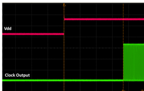
Figure 17. Startup Waveform vs. Vdd
