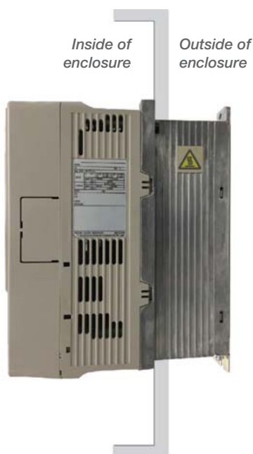
Mounting for external heatsink
