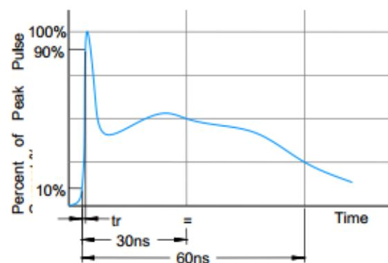
Figure3- 8/20 $\mu$ s Pulse Waveform
