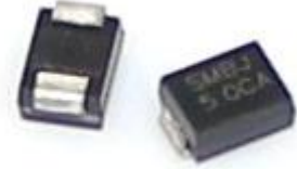
Molded plastic glass passivated junction.
