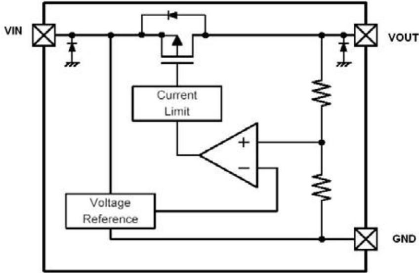
\*Diodes inside the circuit are an ESD protection diode and a parasitic diode.
