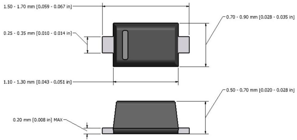
**Note:** Dimensions are exclusive of Burrs, Mold Flash & Tie Bar extrusions.
