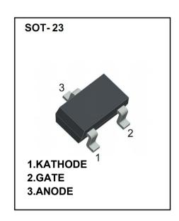
These devices are intened to be interfaced directly to microcontrollers, logic integrated circuits and other low power gate trigger circuits.
