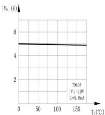
Curve of the output voltage and junction temperature
