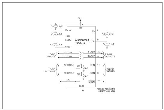
Figure 6. ADM3222A Typical Operating Circuits
