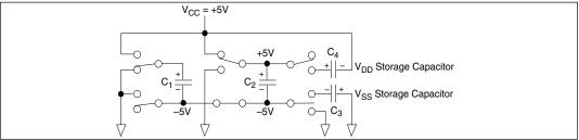
Figure 12. Charge Pump — Phase 1
