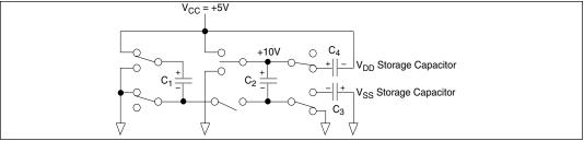
Figure 16. Charge Pump — Phase 4
