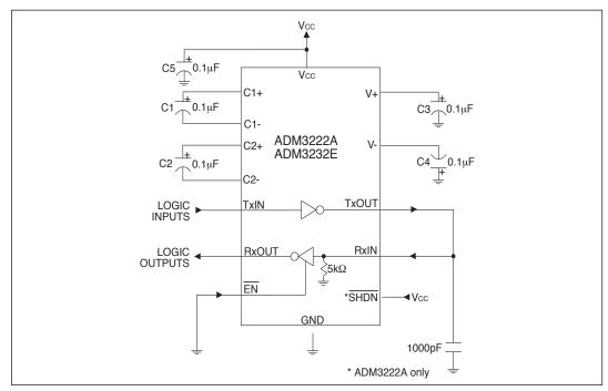
Figure 8. ADM3222A/3232E Driver Loopback Test Circuit
