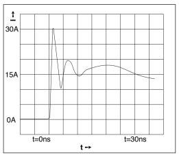
Figure 19. ESD Test Waveform for IEC1000-4-2
