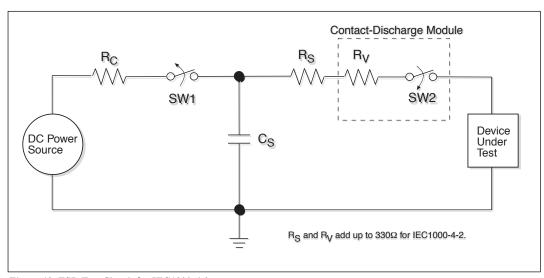
Figure 18. ESD Test Circuit for IEC1000-4-2
