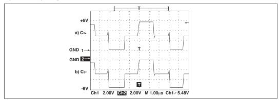
Figure 14. Charge Pump Waveforms
