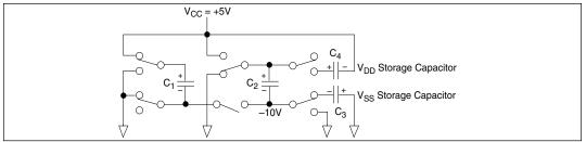
Figure 13. Charge Pump — Phase 2
