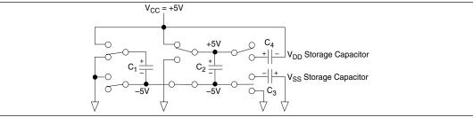
Figure 15. Charge Pump — Phase 3
