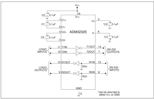
Figure 7. ADM3232E Typical Operating Circuit
