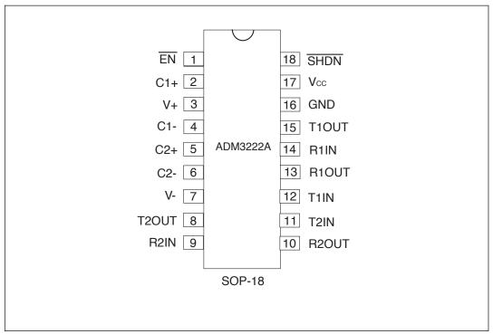
Figure 4. Pinout Configurations for the ADM3222A
