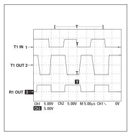
Figure 9. Driver Loopback Test Results at 120kbps
