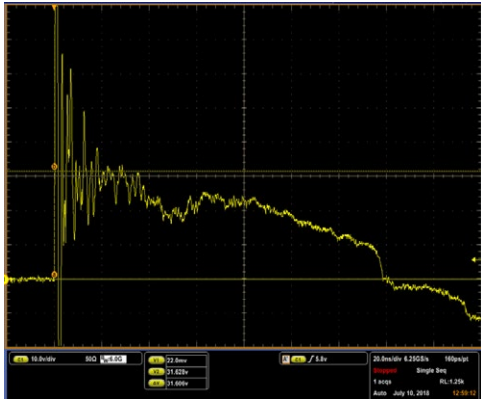
IEC 61000-4-2 +8 kV Contact ESD Clamping Voltage
