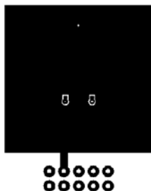
a) 40\text{ }^\circ\text{C/W} when mounted on a 1\text{ in}^2 pad of 2 oz copper
