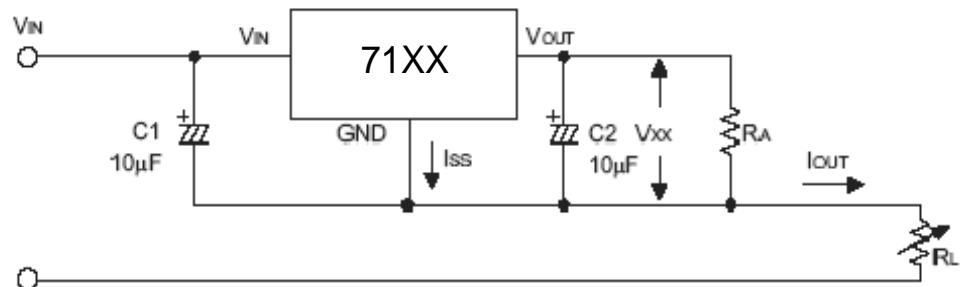
$$I_{OUT} = V_{xx}/R_A + I_{SS}$$
