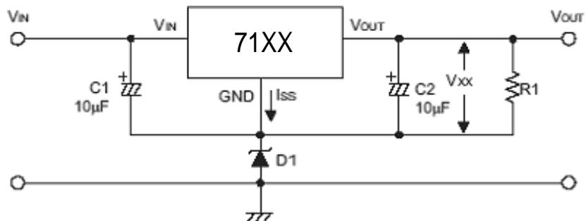
$$V_{OUT} = V_{xx} + V_{D1}$$
