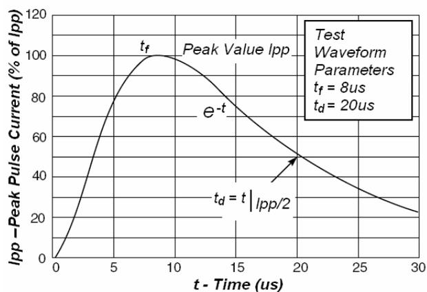
Fig1. Pulse Waveform
