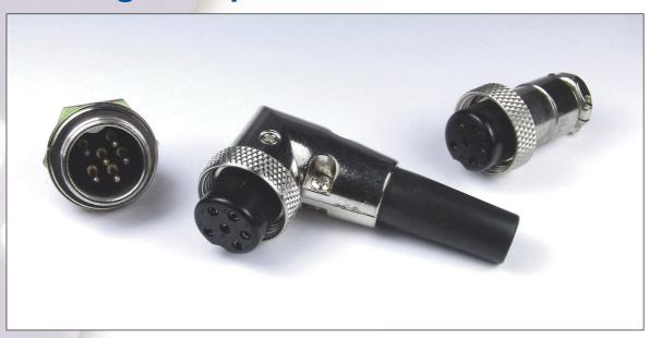
ZC Series are available in a range of 2 pole to 8 pole plugs and sockets. Primarily they are intended for low voltage and signal applications. Contacts are tin plated, and other metal parts are brass or mazac, nickel plated.
