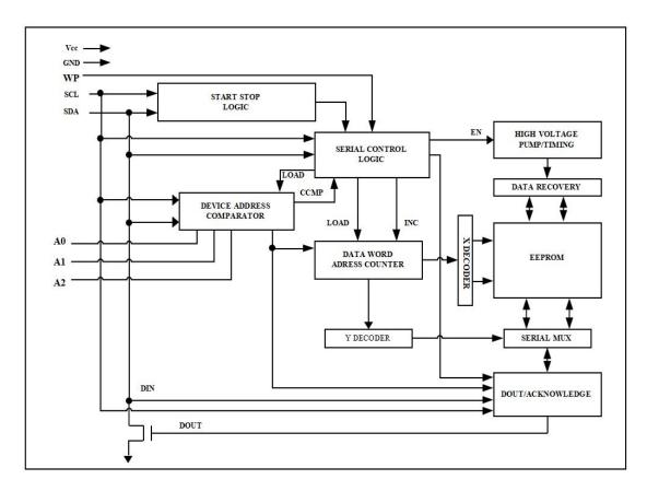
Figure 2-2.System Configuration Using 2-Wire Serial EEPROM
