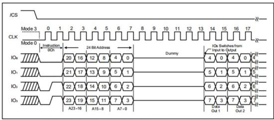
Figure 36b. Burst Read with Wrap instruction (QPI Mode, 108MHz)
