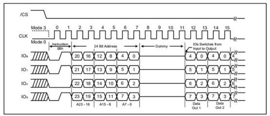
Figure 13b. Fast Read instruction (QPI Mode, 80MHz)
