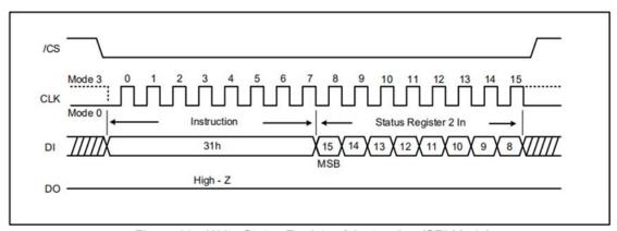
Figure 11a. Write Status Register-2 Instruction (SPI Mode)
