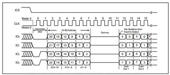
Figure 36a. Burst Read with Wrap instruction (QPI Mode, 80MHz)
