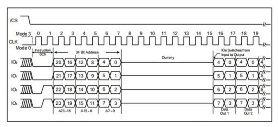
Figure 36c. Burst Read with Wrap instruction (QPI Mode, 133MHz)
