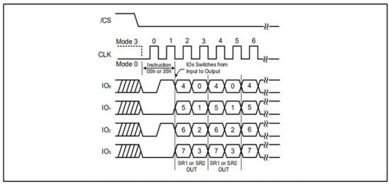
Figure 9b. Read Status Register Instruction (QPI Mode)
