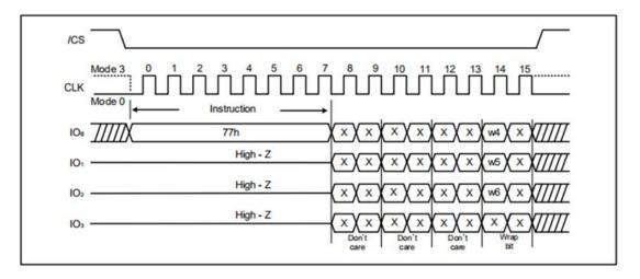
Figure 35. Set Burst with Wrap Instruction Sequence
