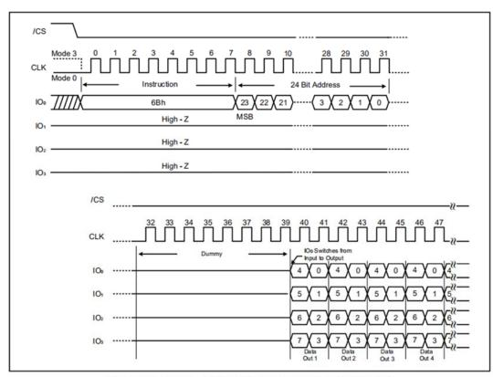
Figure 15. Fast Read Quad Output instruction (SPI Mode)
