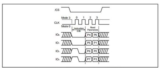
Figure 37. Set Read Parameters instruction (QPI Mode)
