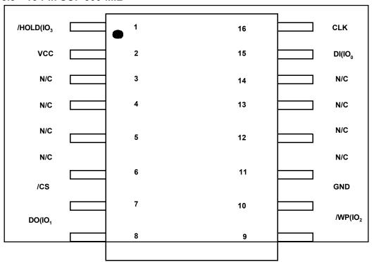
Figure 1c. Pin Assignments, 16-pin SOP 300-mil
