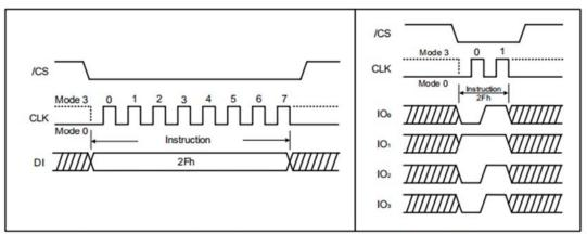
Figure 43. Write Security Register instruction for SPI Mode (left) and QPI Mode (right)
