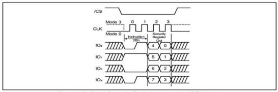
Figure 42b. Read Security Register instruction (QPI Mode)
