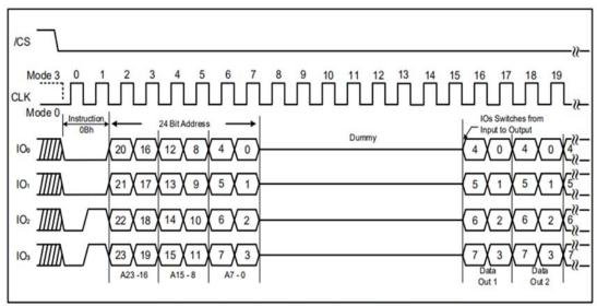
Figure 13d. Fast Read instruction (QPI Mode, 133MHz)
