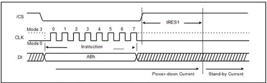
Figure 27a. Release power-down Instruction (SPI Mode)
