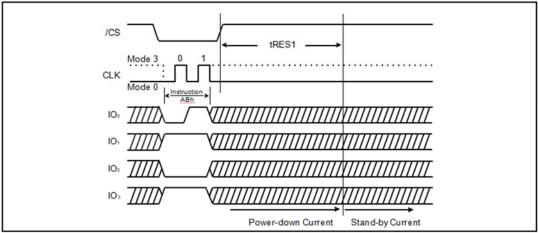
Figure 27b. Release power-down Instruction (QPI Mode)
