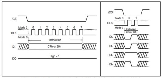
Figure 23. Chip Erase Instruction for SPI Mode (left) and QPI Mode (right)
