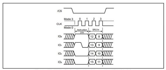
Figure 11b. Write Status Register-2 Instruction (QPI Mode)
