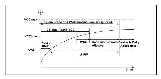
Figure 44. Power-up Timing and Voltage Levels
