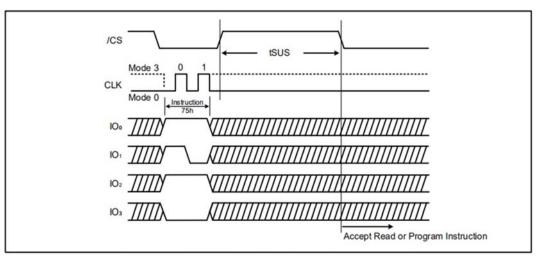
Figure 24b. Erase Suspend instruction (QPI Mode)
