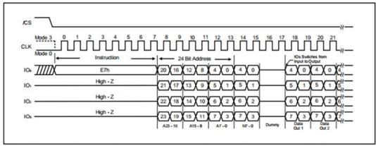
Figure 34a. Word Read Quad I/O instruction (Initial instruction or previous set M7-0 ≠ Axh, SPI Mode)
