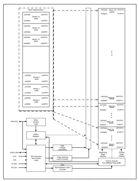
Figure 2. Block Diagram of ZD25Q64B
