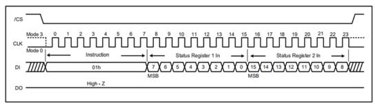
Figure 10a. Write Status Register Instruction (SPI Mode)
