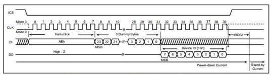
Figure 27c. Release power-down / Device ID Instruction (SPI Mode)
