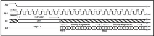
Figure 42a. Read Security Register instruction (SPI Mode)
