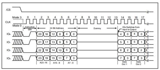
Figure 13c. Fast Read instruction (QPI Mode, 108MHz)
