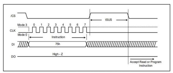
Figure 24a. Erase Suspend instruction (SPI Mode)
