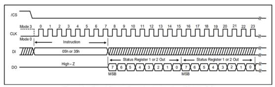
Figure 9a. Read Status Register Instruction (SPI Mode)
