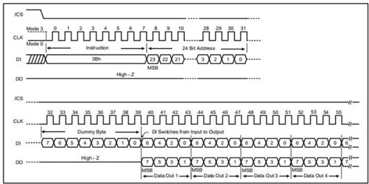
Figure 14. Fast Read Dual Output instruction (SPI Mode)
