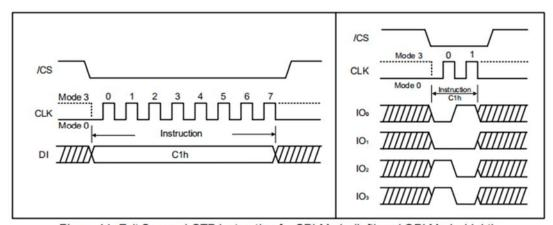
Figure 41. Exit Secured OTP instruction for SPI Mode (left) and QPI Mode (right)
