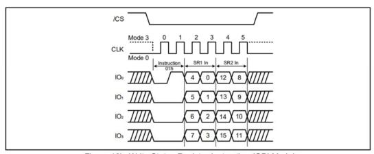
Figure 10b. Write Status Register Instruction (QPI Mode)
