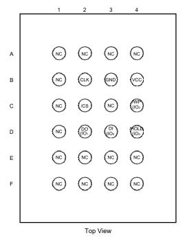
Figure 1d. Pin Assignments, 24-Ball TFBGA
