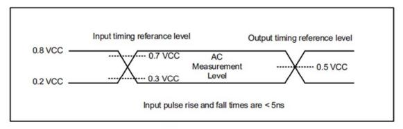
Figure 45. AC Measurement I/O Waveform
