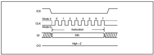
Figure 32. Enable QPI instruction (SPI Mode only)
