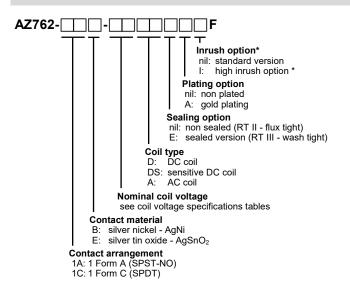
High inrush option only available for 1 Form A (SPST-NO) types with non plated silver tin oxide contacts and standard DC coils.
