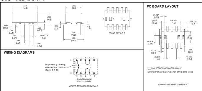
Dimensions in inches with metric equivalents in parentheses. Tolerance: ± .010"
