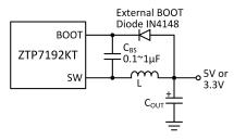
Figure 2: Add optional external bootstrap diode to enhance efficiency.
