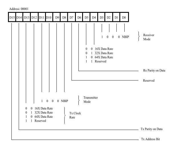
Figure 40. Channel Mode Register, NBIP Mode
