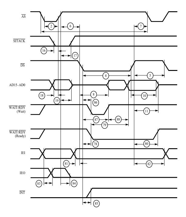
Figure 18. Multiplexed DS Interrupt Acknowledged Cycle
