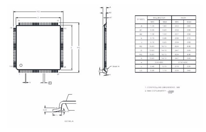
Figure 78. 100-Pin LQFP Package Diagram
