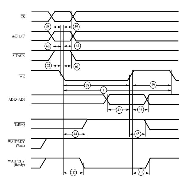
Figure 17. Nonmultiplexed  $\overline{\mbox{WR}}$  Write Cycle
