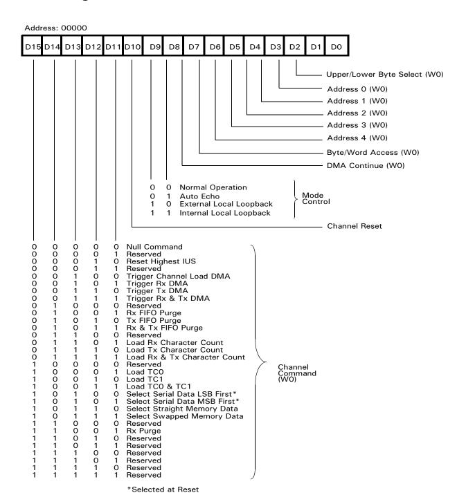
Figure 30. Channel Command/Address Register
