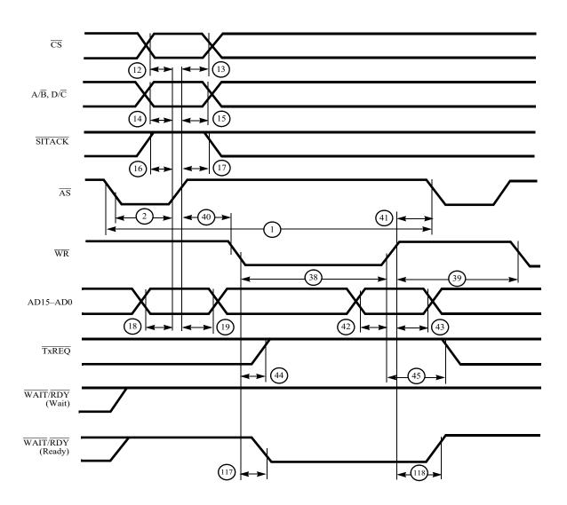
Figure 13. Multiplexed WR Write Cycle
