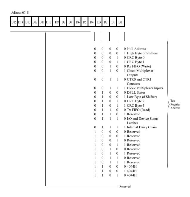
Figure 49. Test Mode Control Register
