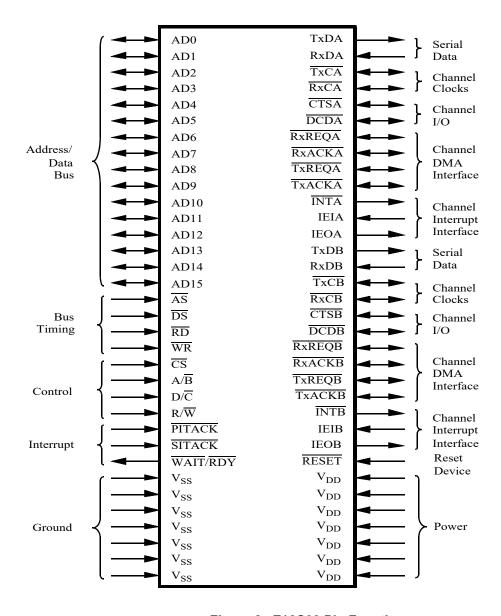
Figure 2. Z16C30 Pin Functions
