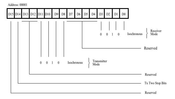
Figure 34. Channel Mode Register, Isochronous Mode
