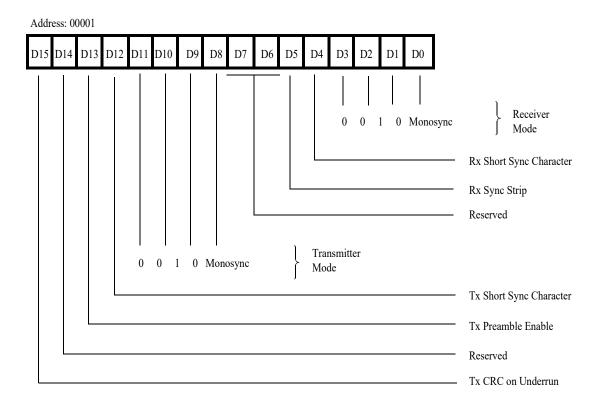
Figure 36. Channel Mode Register, Monosync Mode
