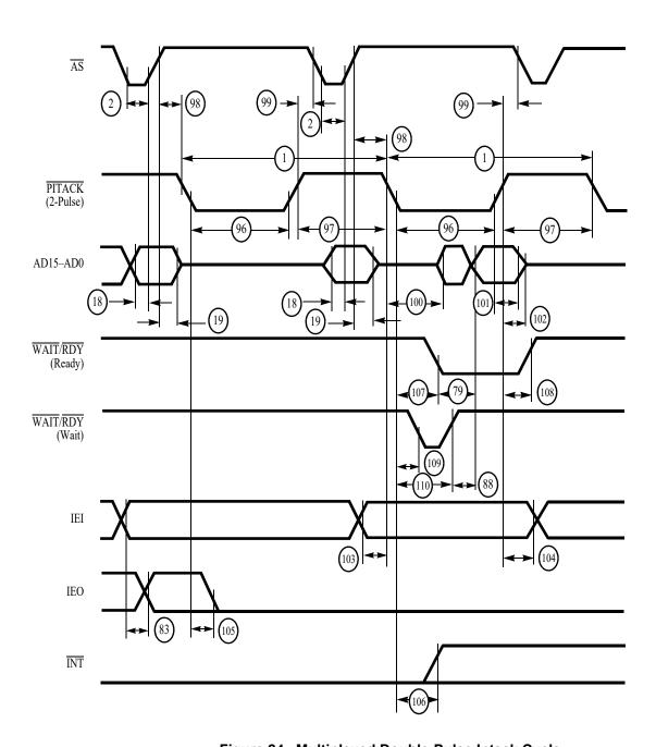
Figure 24. Multiplexed Double-Pulse Intack Cycle
