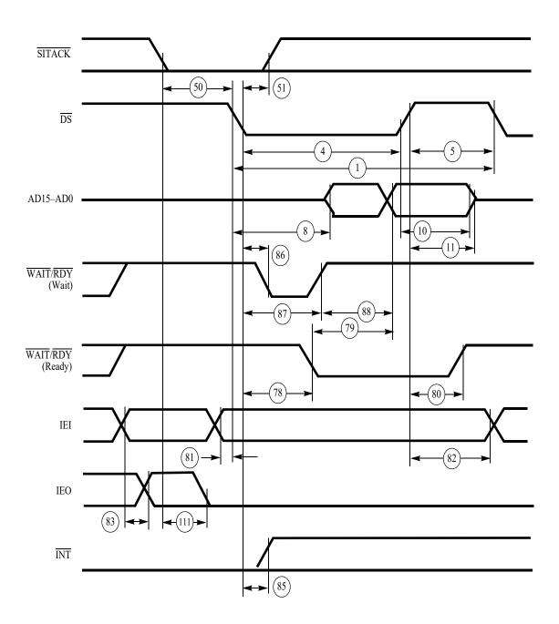
Figure 21. Nonmultiplexed DS Interrupt Acknowledge Cycle
