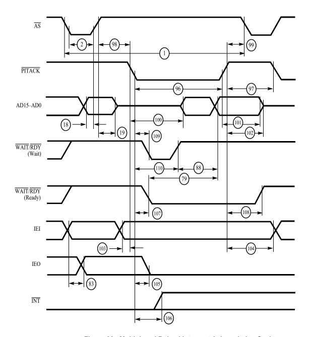
Figure 20. Multiplexed Pulsed Interrupt Acknowledge Cycle
