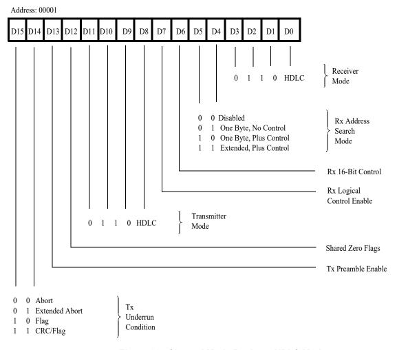
Figure 38. Channel Mode Register, HDLC Mode
