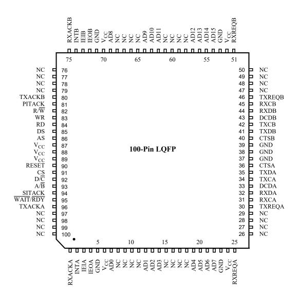
Figure 4. 100-Pin LQFP Pin Assignments
