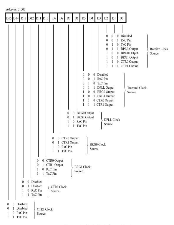
Figure 50. Clock Mode Control Register
