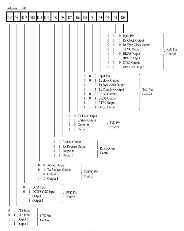
Figure 53. I/O Control Register
