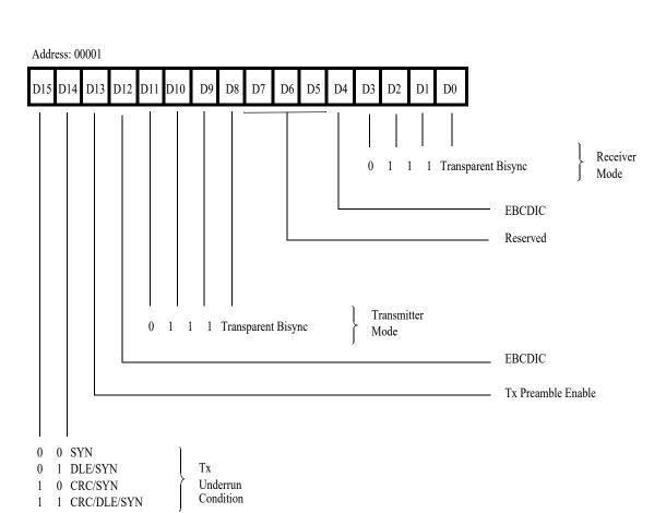
Figure 39. Channel Mode Register, Transparent Bisync Mode
