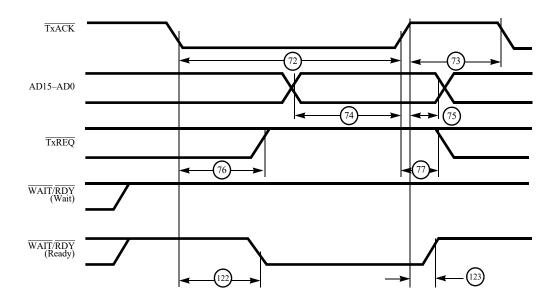
Figure 9. DMA Write Cycle
