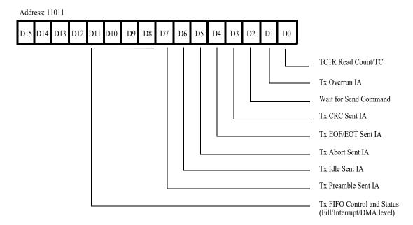
Figure 69. Transmit Interrupt Control Register
