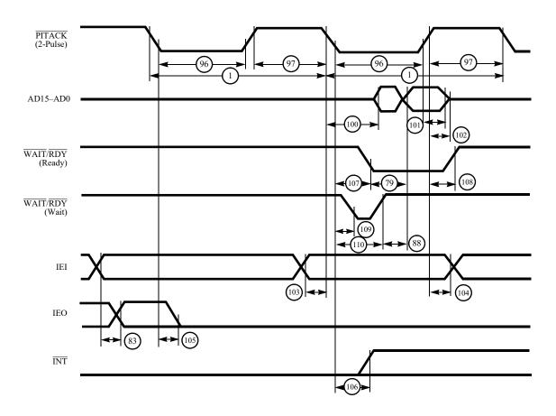
Figure 25. Nonmultiplexed Double-Pulse Intack Cycle
