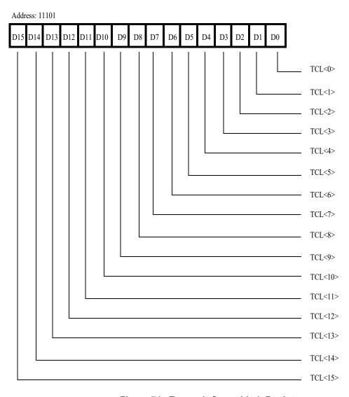
Figure 71. Transmit Count Limit Register
