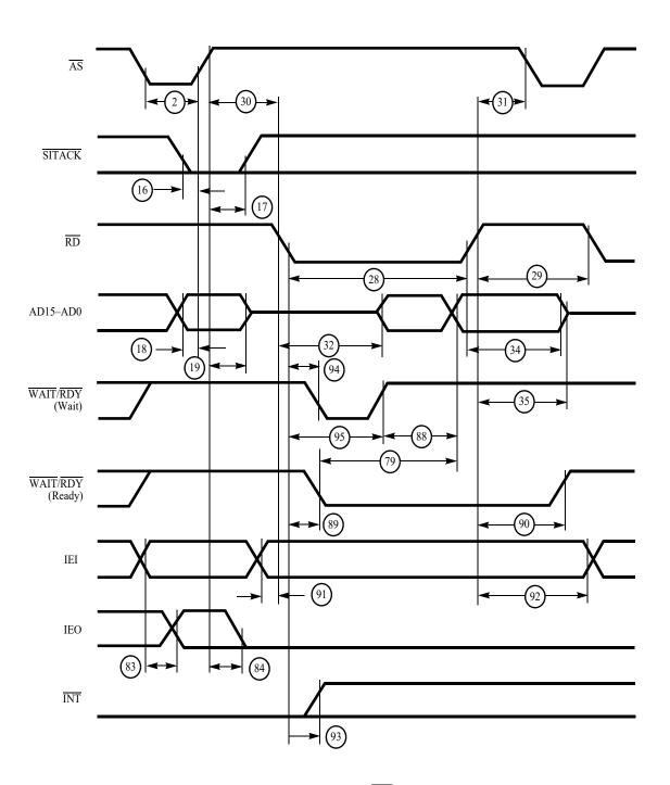
Figure 19. Multiplexed RD Interrupt Acknowledge Cycle
