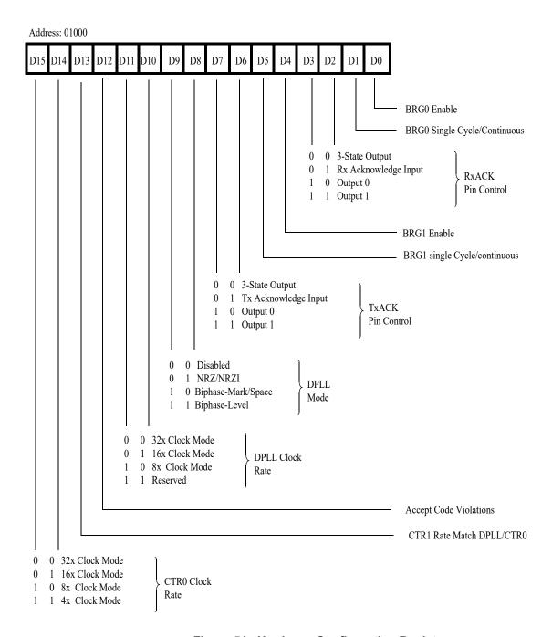
Figure 51. Hardware Configuration Register
