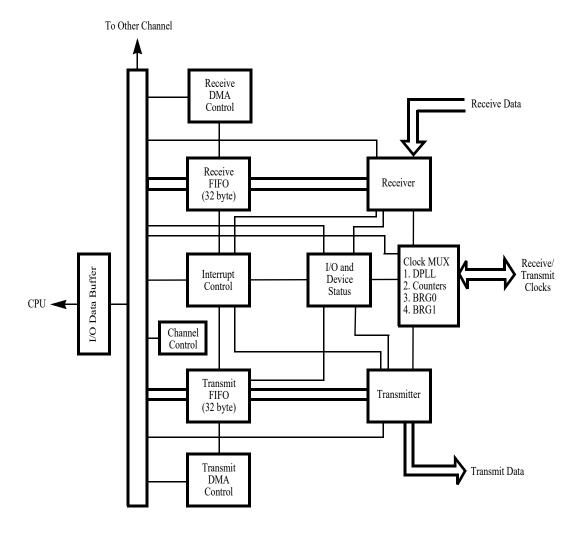
Figure 1. Z16C30 Block Diagram
