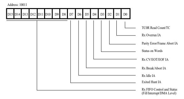
Figure 61. Receive Interrupt Control Register
