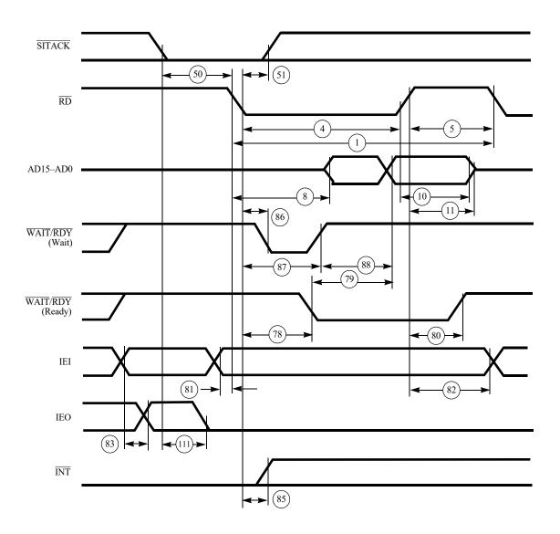
Figure 22. Nonmultiplexed RD Interrupt Acknowledge Cycle
