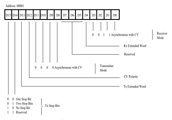
Figure 35. Channel Mode Register, Asynchronous Mode with Code Violation (MIL STD 1553)
