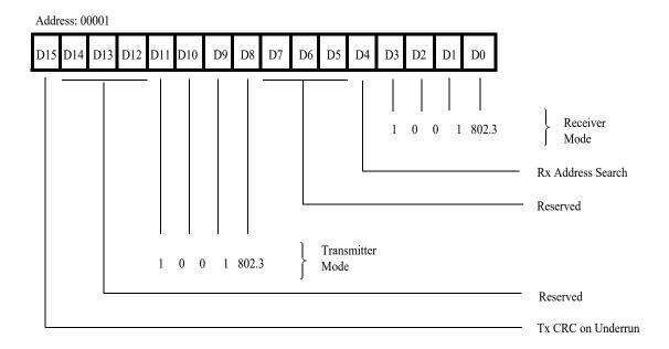
Figure 41. Channel Mode Register, 802.3 Mode
