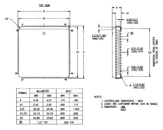
Figure 77. 68-Pin PLCC Package Diagram
