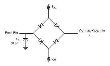
Figure 5. Test Load Diagram
