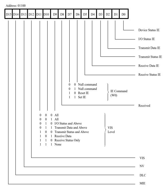
Figure 54. Interrupt Control Register
