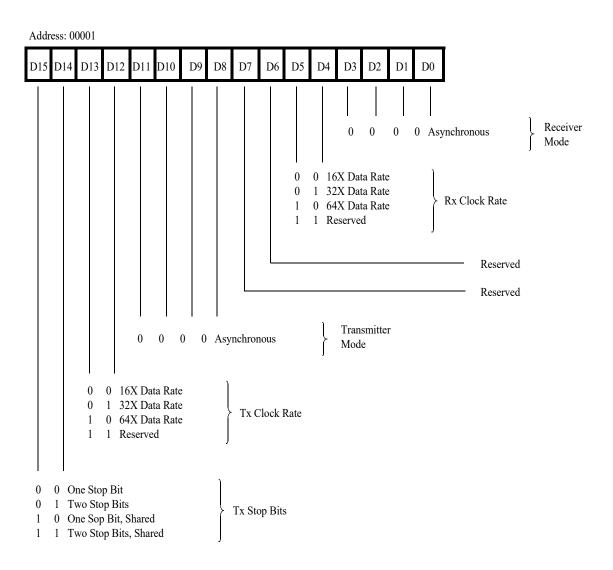
Figure 32. Channel Mode Register, Asynchronous Mode
