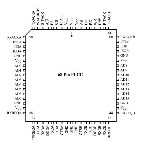
Figure 3. Z16C30 68-Pin PLCC Pin Assignments
