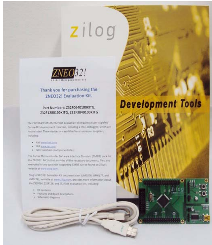
Figure 1. The Z32F128 Evaluation Kit
