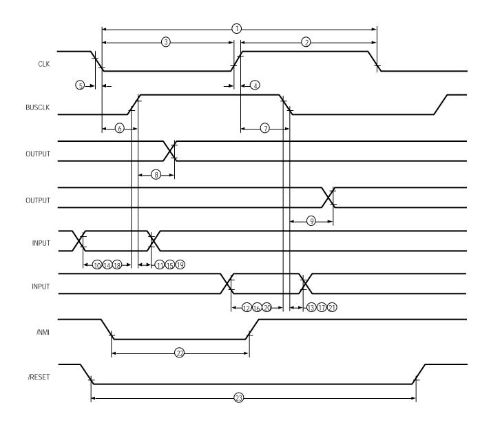
Figure 56. Z380<sup>™</sup> CPU Timing
