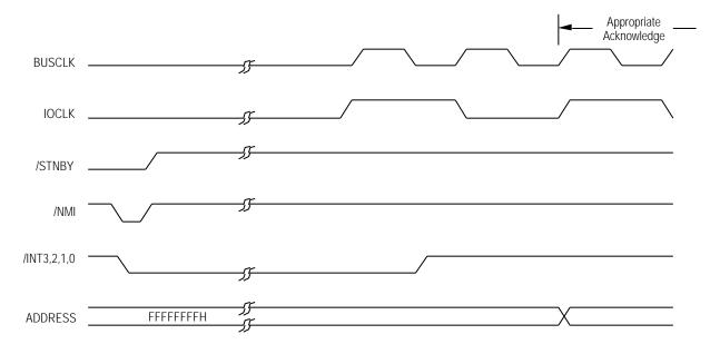
Figure 55. Standby Mode Exit with External Interrupts Timing
