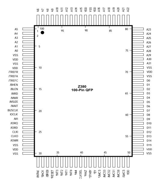
Figure 2. 100-Pin QFP Pin Assignments
