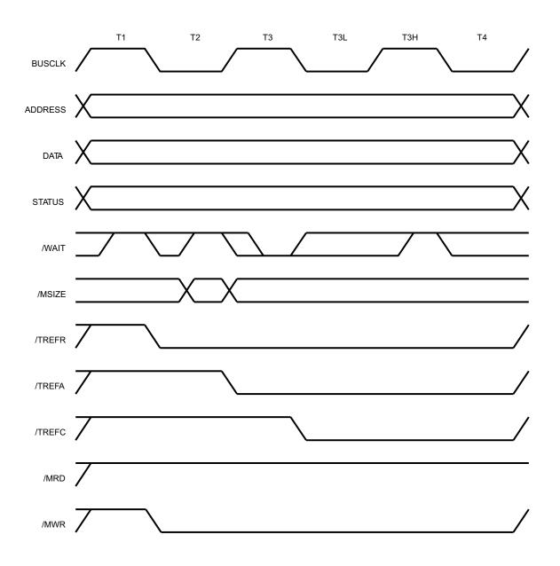
Figure 10. Write Cycle, T3 Wait
