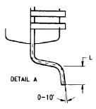
NOTES: 1. CONTROLLING DIMENSIONS : MILLIMETER 2. MAX COPLANARITY : <u>.10</u> .004
