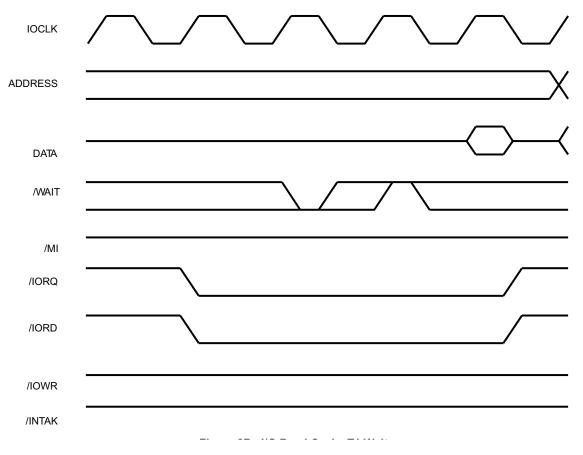
Figure 18. I/O Read Cycle, T1 Wait
