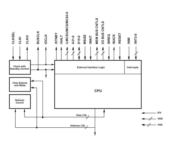
Figure 1. Z380 Functional Block Diagram
