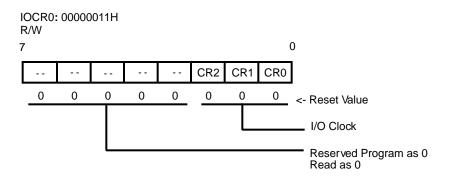
Figure 28. I/O Bus Control Register 0
