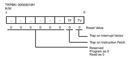
Figure 27. Trap and Break Register
