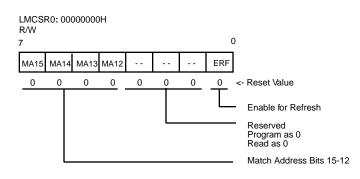
Figure 32. Lower Memory Chip Select Register 0
