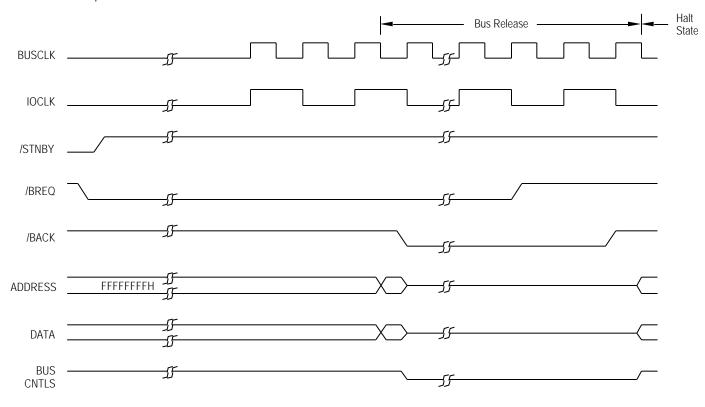
Figure 52. Standby Mode Exit with Bus Request Timing
