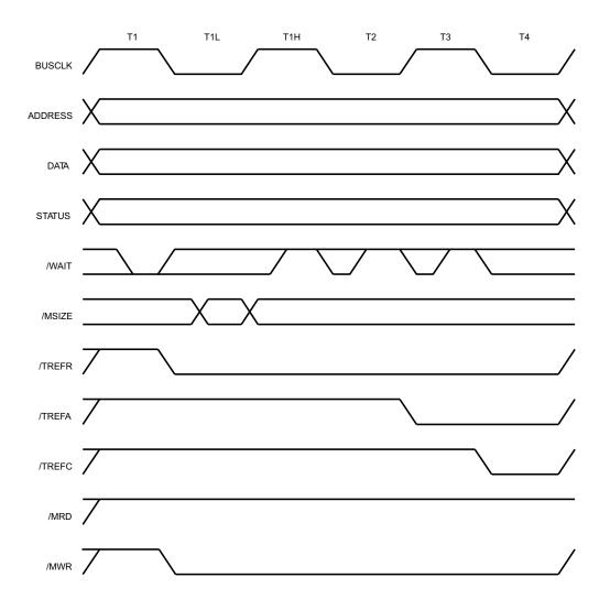
Figure 8. Write Cycle, T1 Wait
