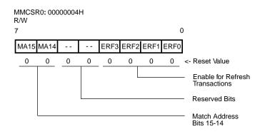
Figure 36. Mid-range Memory Chip Select Register 0
