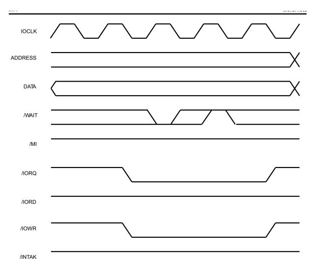
Figure 20. I/O Write Cycle, T1 Wait
