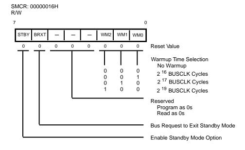
Figure 51. Standby Mode Control Register
