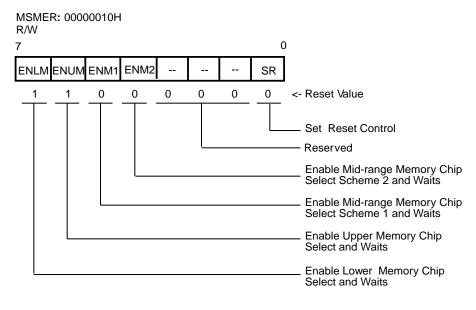
Figure 46. Memory Selects Master Enable Register
