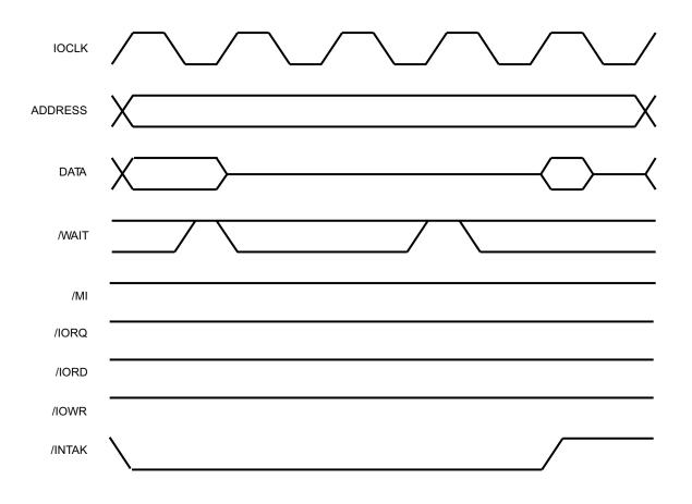
Figure 22. Interrupt Acknowledge Cycle, /INT3-1
