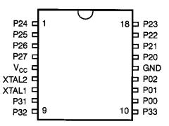
Figure 4. 18-Pin DIP/SOIC Mode Configuration
