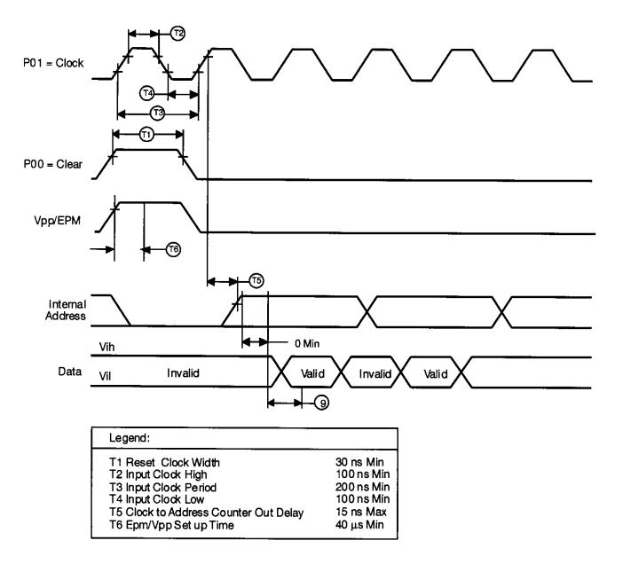
Figure 18. Z86E04/E08 Address Counter Waveform
