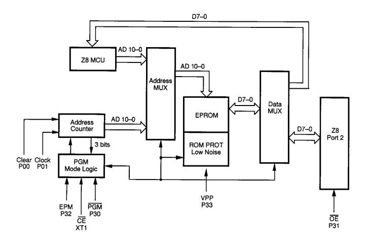
Figure 2. EPROM Programming Mode Block Diagram
