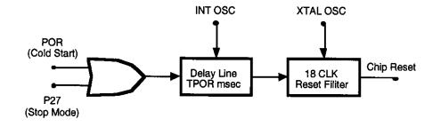
Figure 10. Internal Reset Configuration
