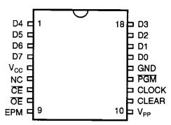
Figure 3. 18-Pin EPROM Mode Configuration
