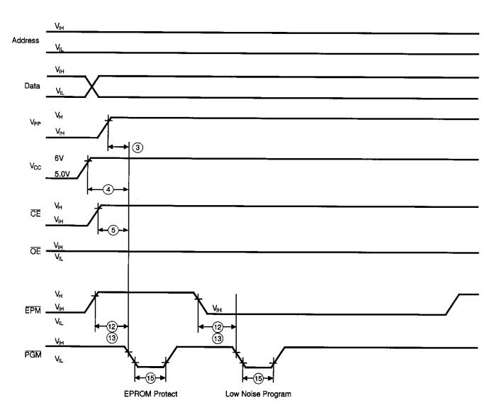
Figure 21. Z86E04/E08 Programming Options Waveform (EPROM Protect and Low Noise Program) Zilog
