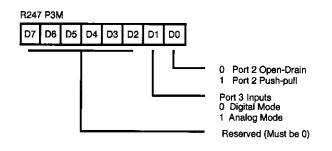
Figure 30. Port 3 Mode Register (F7<sub>H</sub>: Write Only)
