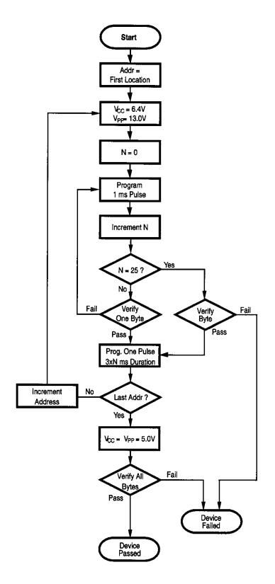
Figure 23. Z86E04/E08 Programming Algorithm
