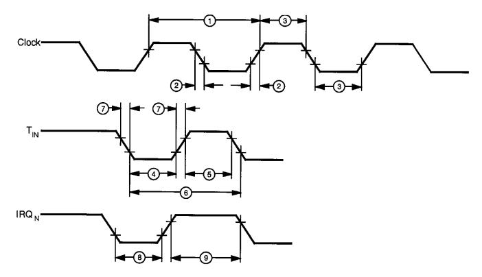
Figure 6. AC Electrical Timing Dlagram
