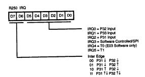
Figure 46. Interrupt Request Register (FA<sub>H</sub>: Read/Write)
