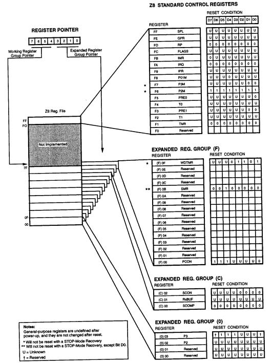
Figure 7b. Expanded Register File Architecture (Z86E06)
