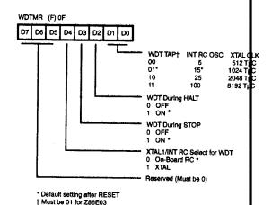
Figure 20. Watch-Dog Timer Mode Register (Write Only)
