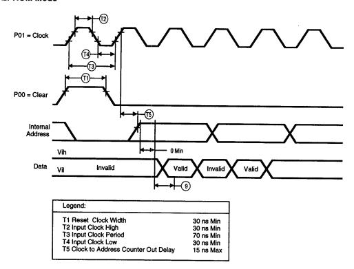
Figure 23. Z86E03/E06 Address Counter Waveform
