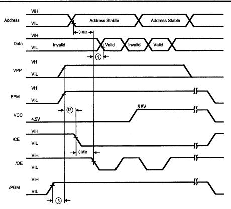
Figure 24. Z86E03/E07 Programming Waveform (EPROM Read)
