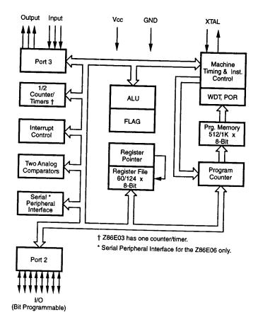
Figure 1. Z86E03/E06 Functional Block Diagram
