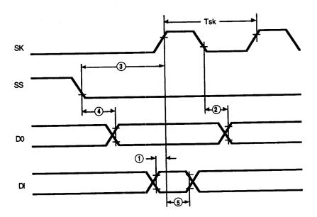
Figure 15. SPI Timing (Z86E06 Only)
