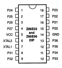
Table 1. 18-Pin DIP and SOIC Pin Identification
