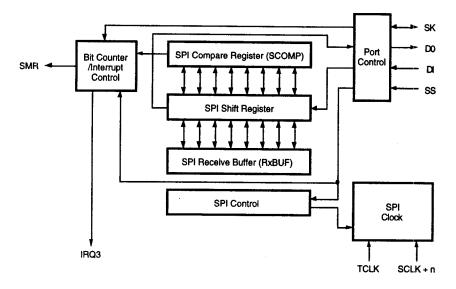
Figure 16. SPI Logic (Z86E06 Only)
