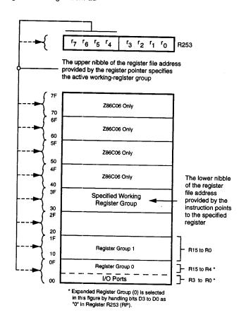
Figure 9. Register Pointer
