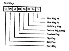
Figure 48. Flag Register (FC<sub>H</sub>: Read/Write)
