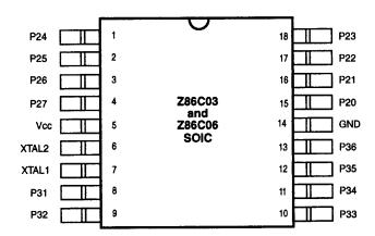
Figure 3. 18-Pin SOIC Pin Configuration
