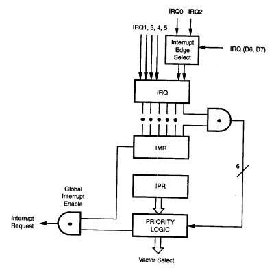
Figure 11. Interrupt Block Diagram
