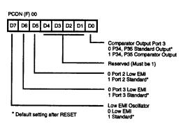
Figure 17. Port Configuration Register (PCON) (Write Only)
