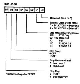
Figure 18a. STOP-Mode Recovery Register (Write Only except bit D7, which is Read Only.) (Z86E03)
