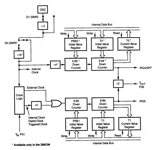
Figure 10. Counter/Timer Block Diagram
