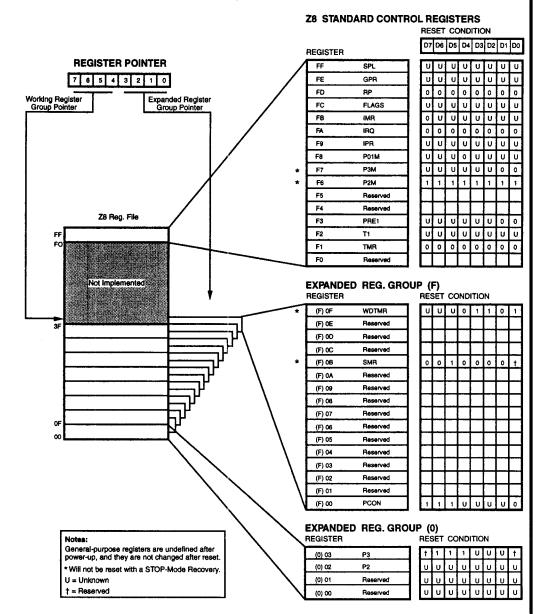
Figure 7a. Expanded Register File Architecture (Z86E03)
