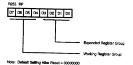
Figure 8. Register Pointer Register
