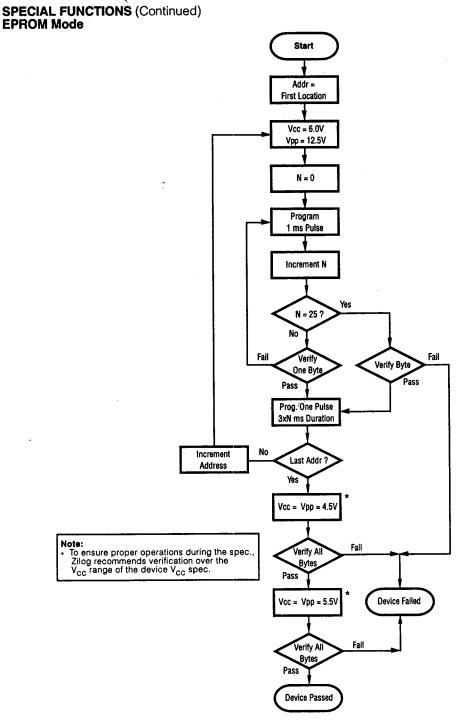
Figure 27. Z86E03/E06 Programming Algorithm
