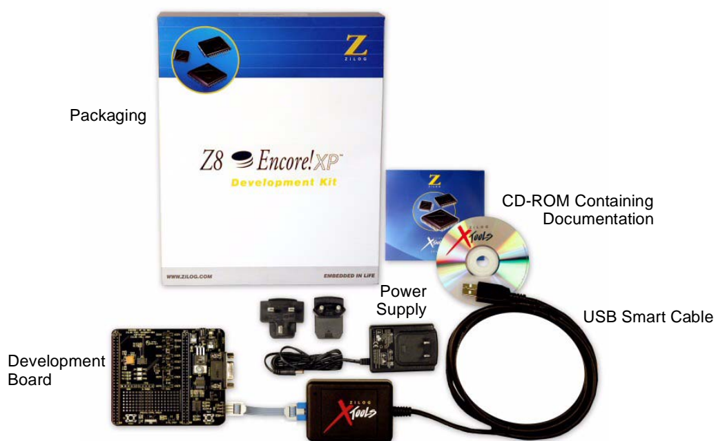
Figure 1. Z8 Encore! XP F042A Series 8-Pin Development Kit Contents (Printed Quick Start Guide Not Shown)
