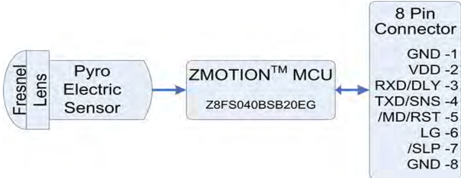
Figure 1. ZMOTION Block Diagram (ZEPIR0AxS02MODG)
