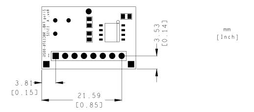
Figure 10. Mechanical Drawing of the ZMOTION Detection Module II (Straight Pins, ZEPIR0BBS02MODG)
