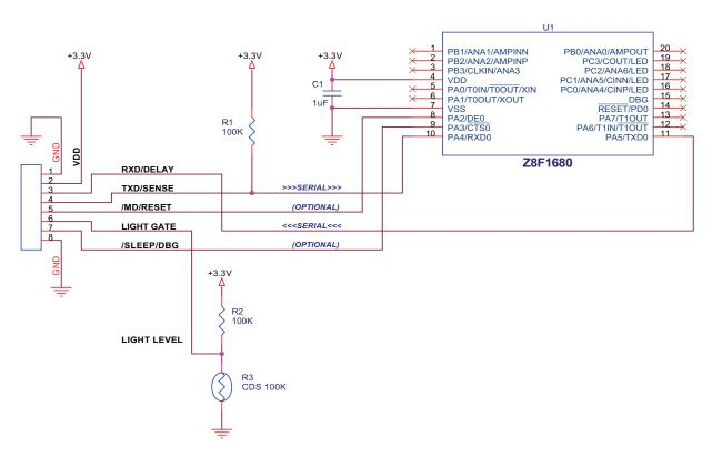
Figure 13. Application Example, Serial Interface Mode
