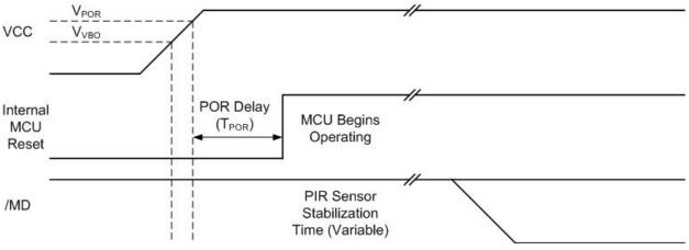
Figure 3. Power-On Reset Operation
