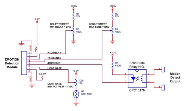
Figure 12. Application Example, Hardware Interface Mode
