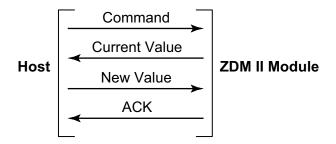
Figure 6. Write Command Structure
