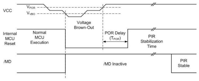
Figure 4. Voltage Brown-Out Reset Operation
